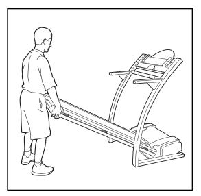
2. Move your right hand to the position shown and hold the treadmill firmly. Using your left hand, pull the latch knob to the left and hold it. Raise the treadmill until the latch pin is aligned with the hole in the catch. Insert the latch pin into the catch. Make sure that the latch pin is fully inserted into the catch.
